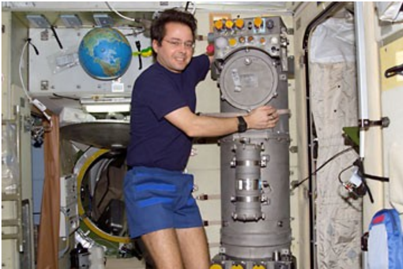
Elektron system on the International Space Station
