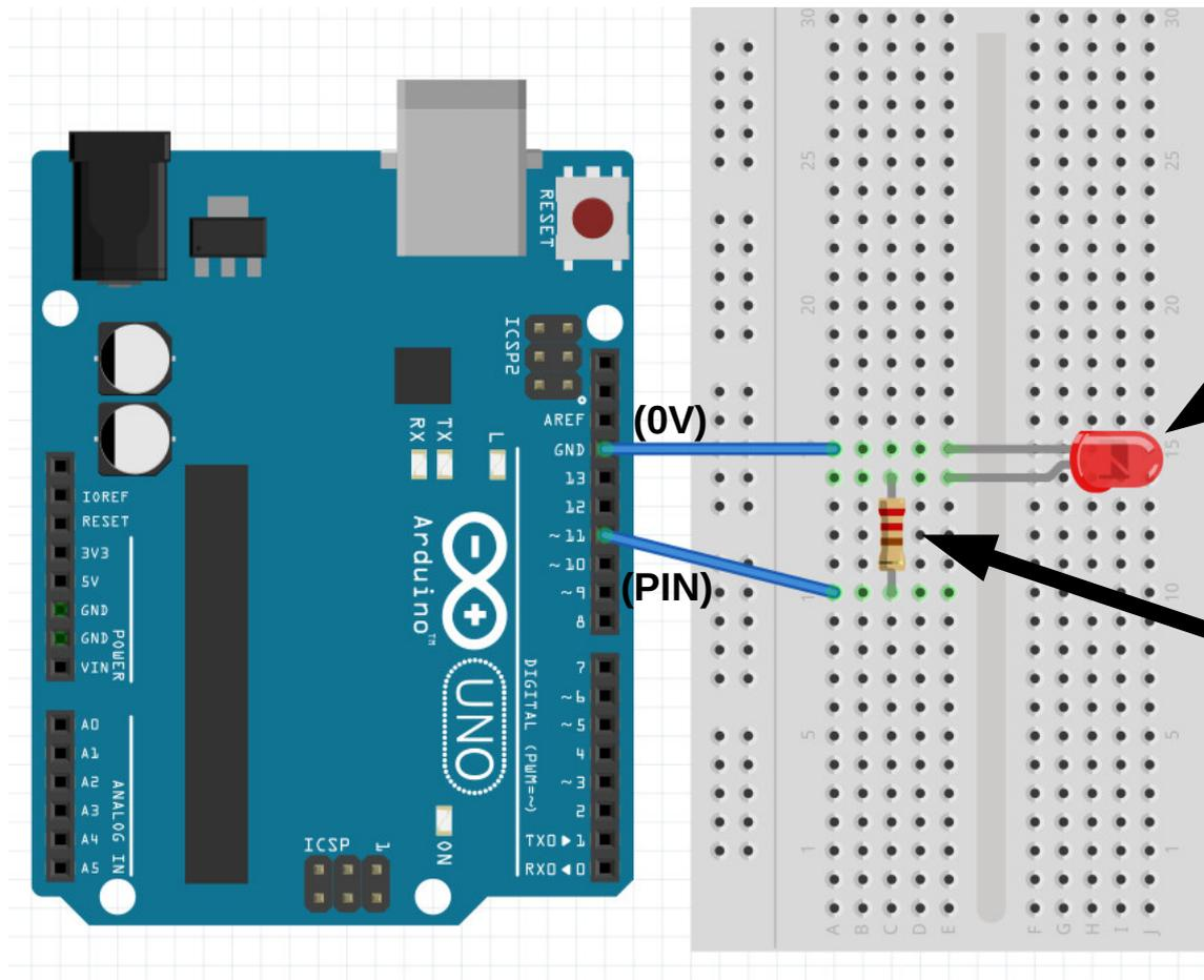
When PIN is set to LOW (0V), there's no voltage differential across circuit, so no current.
