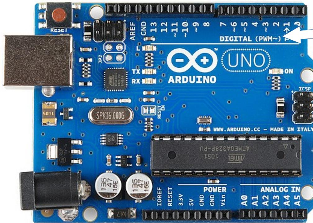
The board usually indicates which pins have PWM built-in support
