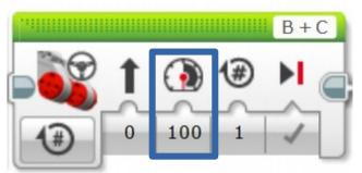
The Large Motor has a <u>top speed</u> of ~2.8 revolutions per second.
