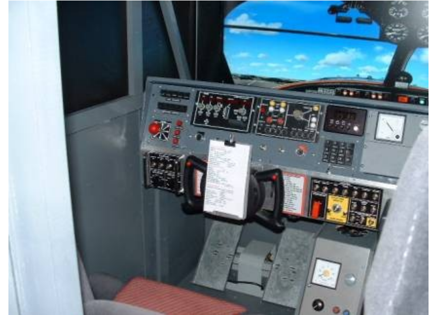
Flight simulator (...this one was built using an Arduino)
