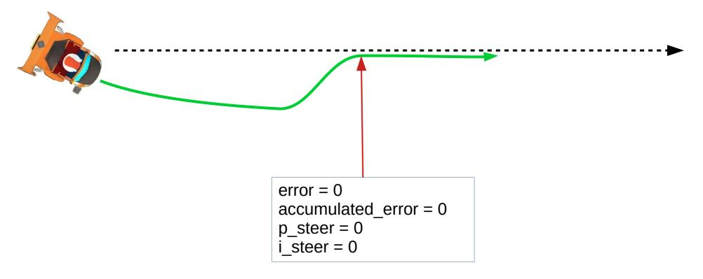
Both error and accumulated\_error are zero, so the the robot go straight
