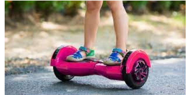
Hoverboards uses a gyro to keep the user upright
